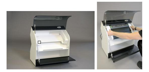
5. Place the paper on the paper shelf. Insert the paper and fit it to both of the tractors located inside of the Basic-D V4 embosser. (For additional paper mounting instructions please see the embosser user manual.)
