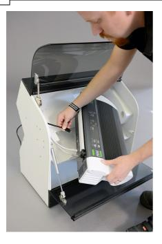
4. Lift the Basic-D V4 embosser into the unit and place it in the fitted embosser grooves located on the embosser shelf.
