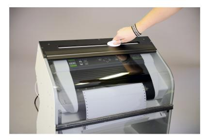
9. Pick up the embossed document from the bottom paper dispense shelf of the unit. (ensure that the paper falls as originally stacked on the paper shelf)
