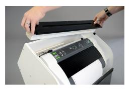
• Remove the remaining two screws of the black profile. Lift off the black profile.
