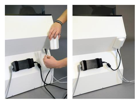
3. Connect all cables into the embosser's electrical connectors by balancing the embosser on the embosser shelf inside the Acoustic unit. (see the embosser user manual for details)
