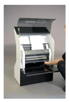
7. Test the paper feed by pressing FEED on the embosser. Test a couple of sheets to ensure a successful feed to the lower shelf of the Hood.
