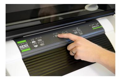
6. Test the paper feed by pressing FEED on the embosser. Test a couple of sheets to ensure a successful feed to the lower shelf of the Hood.
