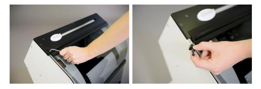
Remove the top part of the hinge connection by pressing downward on the Hinge Lock until the hinge is free from the glass.
