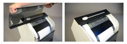
Using the supplied 3 mm Allen Key, remove the black profile and cutting mechanism module by removing three screws (see picture).
