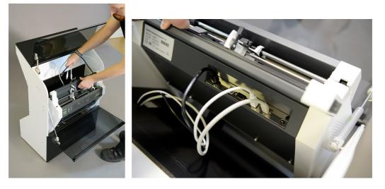
5. Place the paper in the embosser's sheet feeder. Insert the paper according to the orientation of your document. Additional paper setting details may be found in the embosser user manual.
