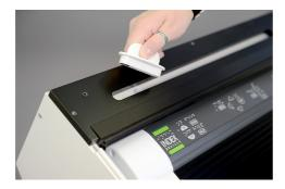
• Lift upward to remove the cutting mechanism module
