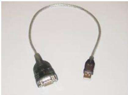
Figure 2: RS232 to USB converter 1
