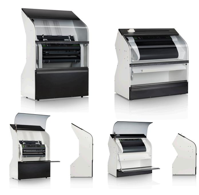
The **Everest Hood V4/V5** supports paper sizes up to A3 or 11X17 inch paper, reduces the noise level to 58 dB(A) and holds a full sheet-feeder of about 50 sheets of paper.
