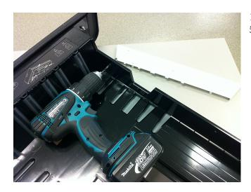
11. Remove the paper guide and expand the two holes using a 5.5 mm speed drill.
