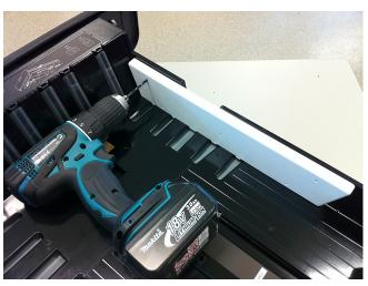
10. Place the guides in position. Drill through the two TOP holes using a 4mm speed drill.
