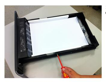
19. Place your paper in the tray and adjust the paper guides using a PH2 screwdriver.
