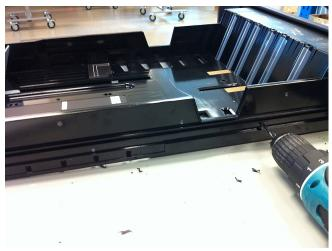
$14.\ Remove$  the paper guide and expand the three holes using the  $5.5\ mm$  speed drill.
