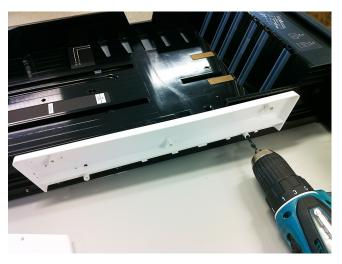
13. Drill the three remaining holes using the 4 mm speed drill.
