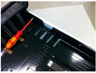
12. Mount the paper guide on the outside with two screws (5.0 x 16)  $\,$
