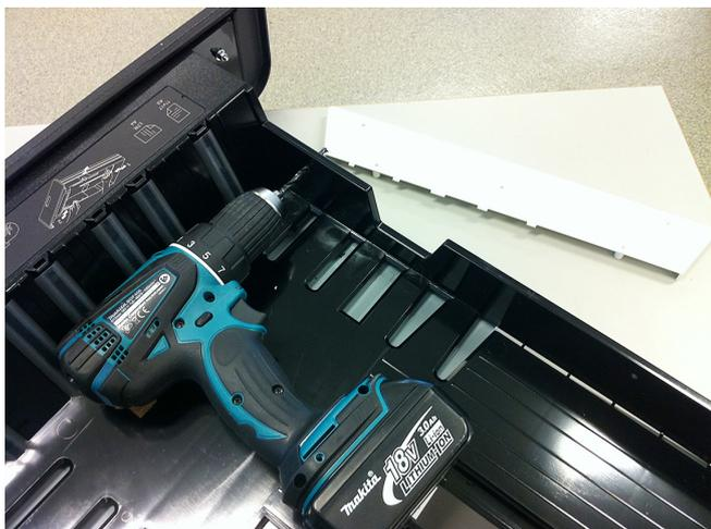
11. Remove the paper guide and expand the two holes using a 5.5 mm speed drill.
