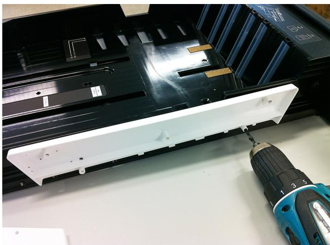
13. Drill the three remaining holes using the 4 mm speed drill.
