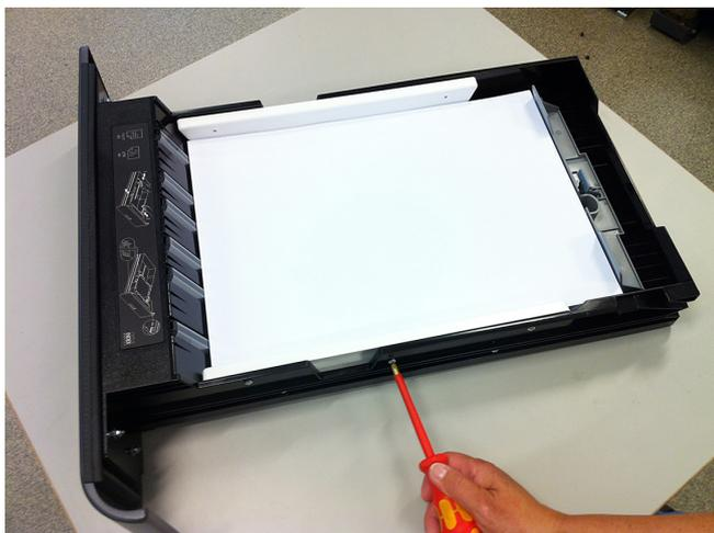
19. Place your paper in the tray and adjust the paper guides using a PH2 screwdriver.
