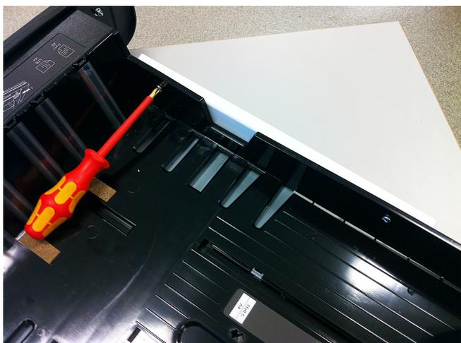
12. Mount the paper guide on the outside with two screws (5.0 x 16)
