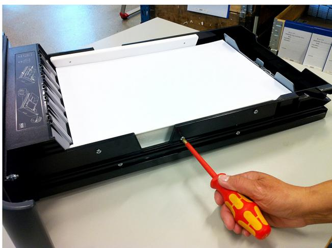
20. Adjust the Paper guides so that the paper is centered in the tray. Do not overtighten the guides, the paper should slide smoothly up to the embossing tower.
