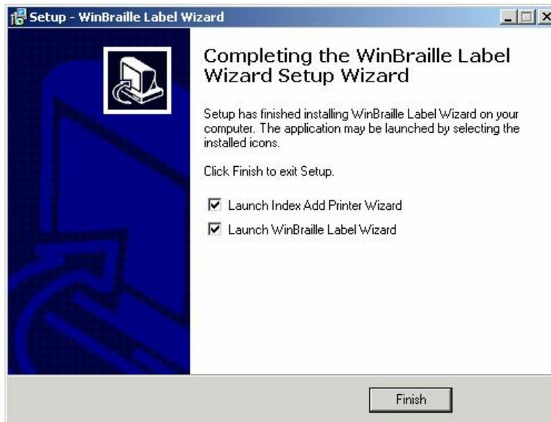
To install an Index Braille embosser to use for the Label printouts keep the selection **Launch Index Add printer Wizard** checked. If the embosser that you are going to use is installed already, uncheck it.
